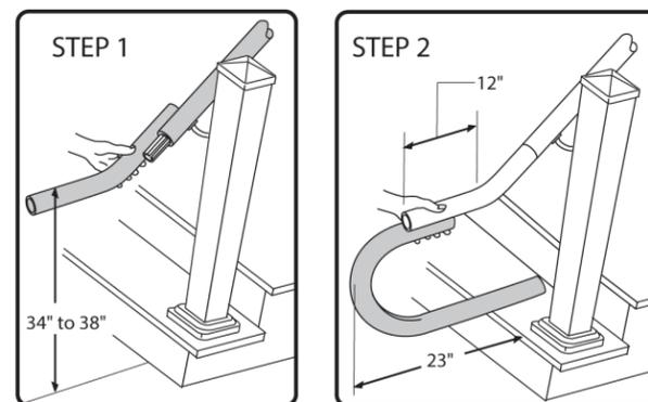
With corner now in place, determine the height of the in-line brackets on a step railing installation by holding a piece of railing in line with the elbow and parallel to the primary railing.
