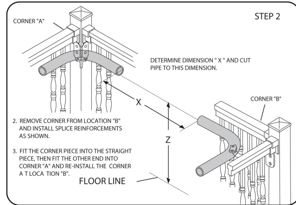
Where ever two ends of aluminum ADA handrail are joined, either to each other or to elbows, tighten the joint by drilling a 9/32" countersink and 5/32" thru hole and securing with screws. Make sure screw heads are smooth. (See next page, Finishing Connections)
